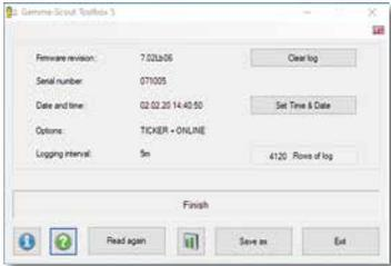
2. Raw data files from an ONLINE model with firmware 7.02 or newer can be saved and loaded again later without the device. The **bar-chart icon** also appears with loaded raw data.
