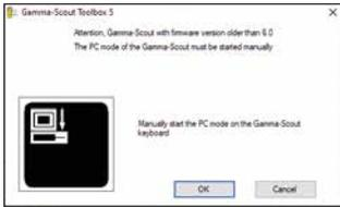
2. The data transfer will take longer with an older GAMMA-SCOUT® model. Another toolbox dialog opens when the upload is complete.
