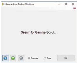
2. Connect the GAMMA-SCOUT® to your computer using the cable supplied. The software establishes a connection with the GAMMA-SCOUT®. This can take a few seconds.
