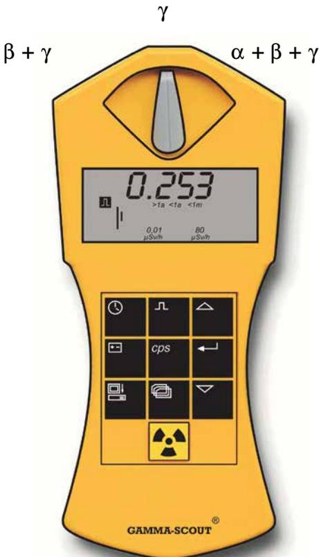
To measure environmental radiation, you should have the radiation selection switch in the middle position.  $\alpha$  and  $\beta$  radiation have short ranges or just a few centimeters or meters and are therefore encountered only in the immediate vicinity of the radiation sources.
