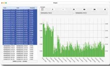
The values selected in the table are shown in the bar chart. Click on a row in the table. Hold the mouse button and move the cursor to select the desired table section. Release the mouse button.
