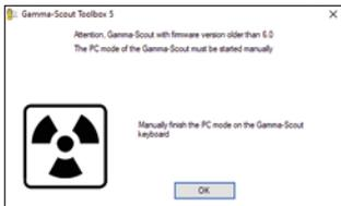
3. Press the **Radiation reading** button on the GAMMA-SCOUT® and click **OK** in the Toolbox dialog that appears.
