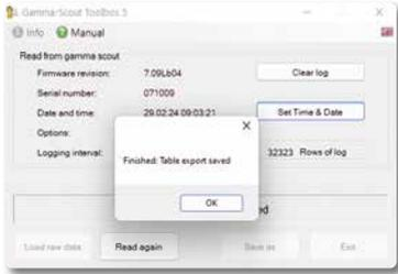
7. Click **Set Date & Time** to overwrite the internal GAMMA-SCOUT® clock with the current date and time from your system.
