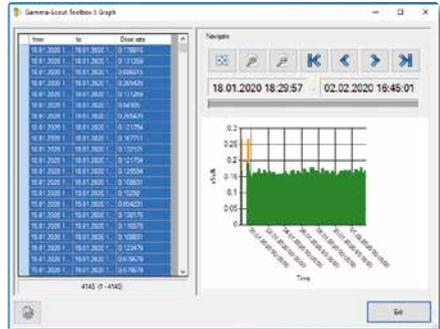
5. The values selected in the table are shown in the bar chart. Click on a row in the table. Hold the mouse button and move the cursor to select the desired table section. Release the mouse button. The selected table rows are displayed as a bar chart. The X axis represents the measurement time period. The Y axis shows the level of the dose rates as colored bars.
