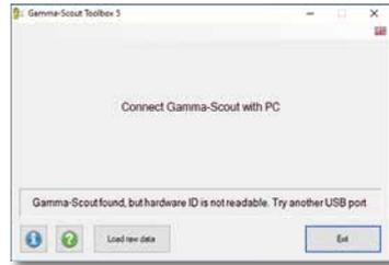
Windows 10 sometimes uses a different USB driver than the one installed with Toolbox 5. This depends on the Windows 10 security settings. The GAMMA-SCOUT® has no control over these settings. An incorrect USB driver often causes timeout errors when reading out the data. The Toolbox checks whether an incorrect driver is being used and then displays an error message.
