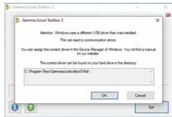
The user has to find the correct driver in the Windows 10 Device Manager and assign it to the GAMMA-SCOUT® connection. The folder with the correct driver files is displayed in the screen dialog.
