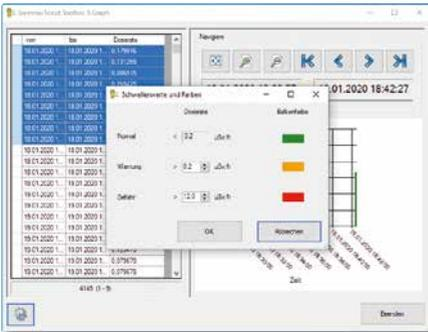
You can set two limits for the dose rate on the left. Set the desired bar colors on the right.
